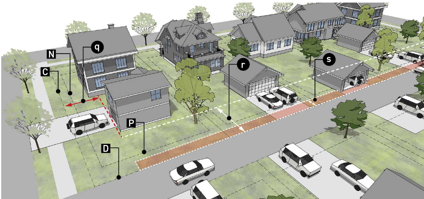
FIG. 15 Alley and Side Access Setbacks
